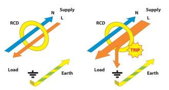
The device monitors the ingoing and outgoing current flow and trips when an imbalance occurs as illustrated above.
